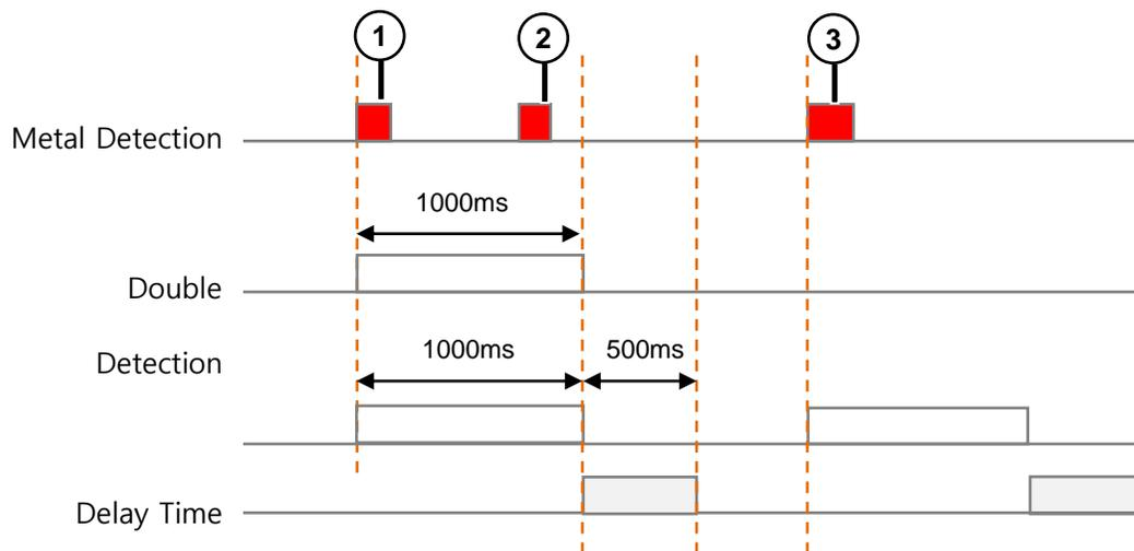
In the above picture, in the point where the metal ① is detected, if the metal ② passes during the double detection time 1000ms, the metal is not detected. Within the double detection time, the two would be detected as one.
