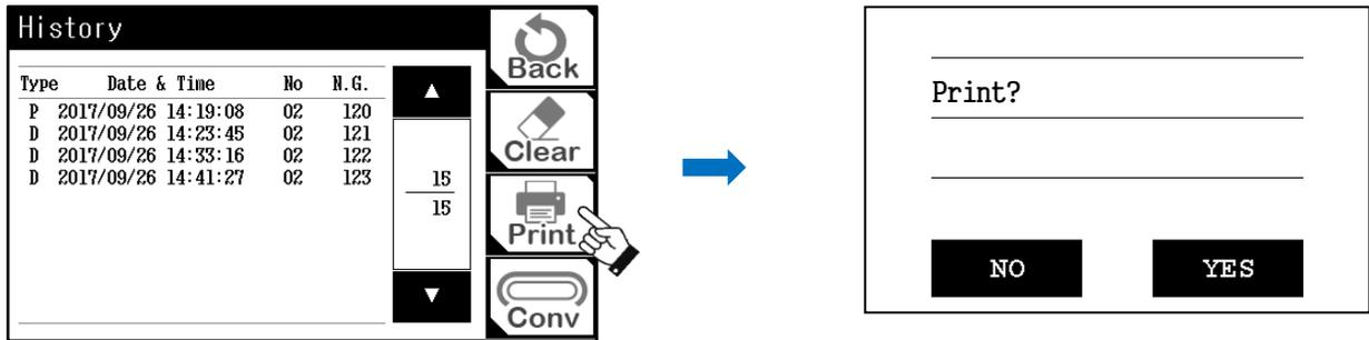
By pressing the [Print] button, the installed printer prints out the content of the detection history.
